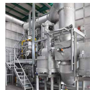
PulsReg®-Zentral Pulsed regenerative burner system
