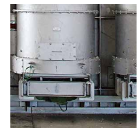
RegClean® (option) Cleaning system for regenerators
