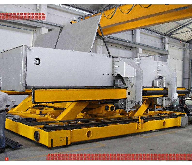
Movable — for charging contaminated scrap to hearth and multi-chamber melting furnaces with closed charging trough and hood
