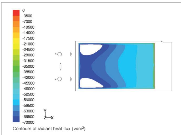
**Fig. 5:** Radiative heat transfer into the aluminium bath (low impulse)
