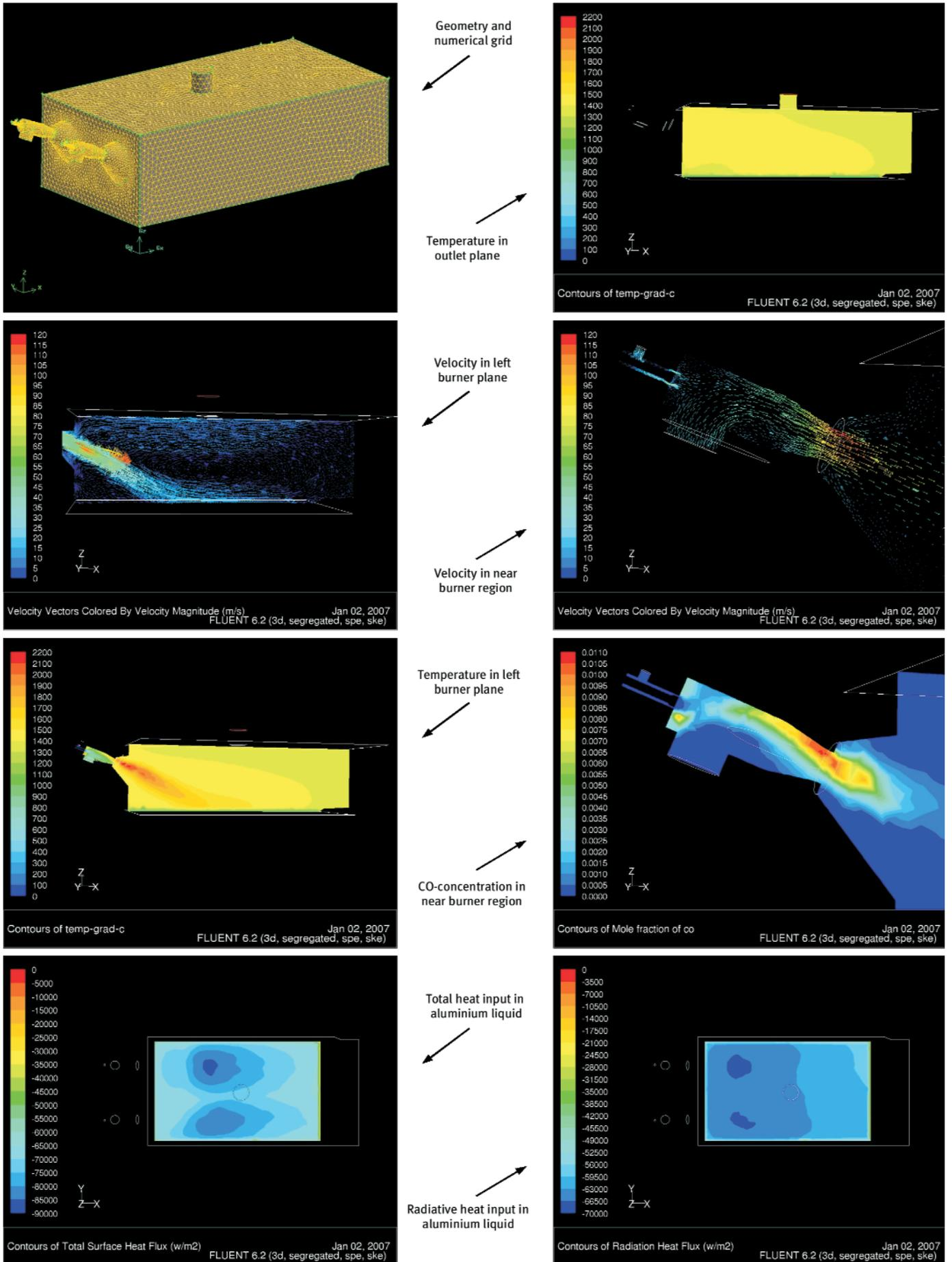
Fig. 1: Numerical simulation of an aluminium melting furnace
