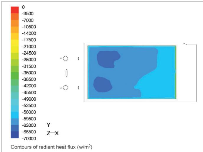
**Fig. 4:** Radiative heat transfer into the aluminium bath (high impulse)
